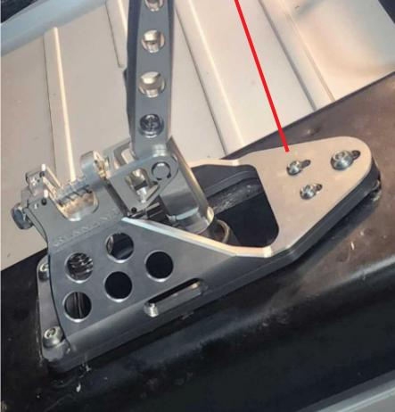
When tightening these two up you want to align the bottom center screw up with the hole so when you inset and tighten the shifter down the screw goes through the carrier plate and does not bend it.
