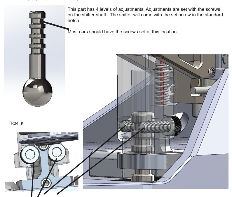
Remove screws to fully adjust.
