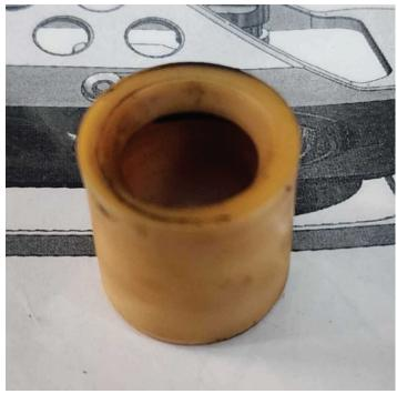
As well, the Shift Rod Bushing should be inspected for damage or is worn.
