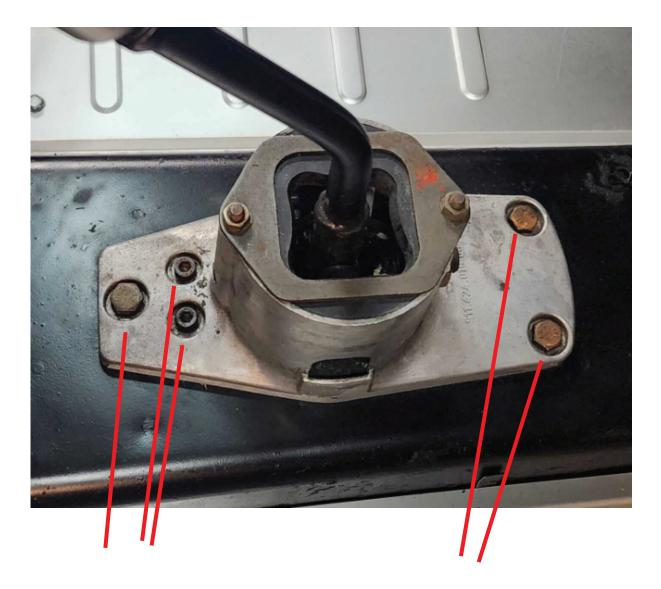
Start this installation by removing these bolts and these Hex head screws. Once removed you can pull upwards to remove the shifter end from it's socket. Please note that over time this cup can be stuck inside and become difficult to remove. If you are not careful the shifter can release very quickly and damage interior parts of the car.
